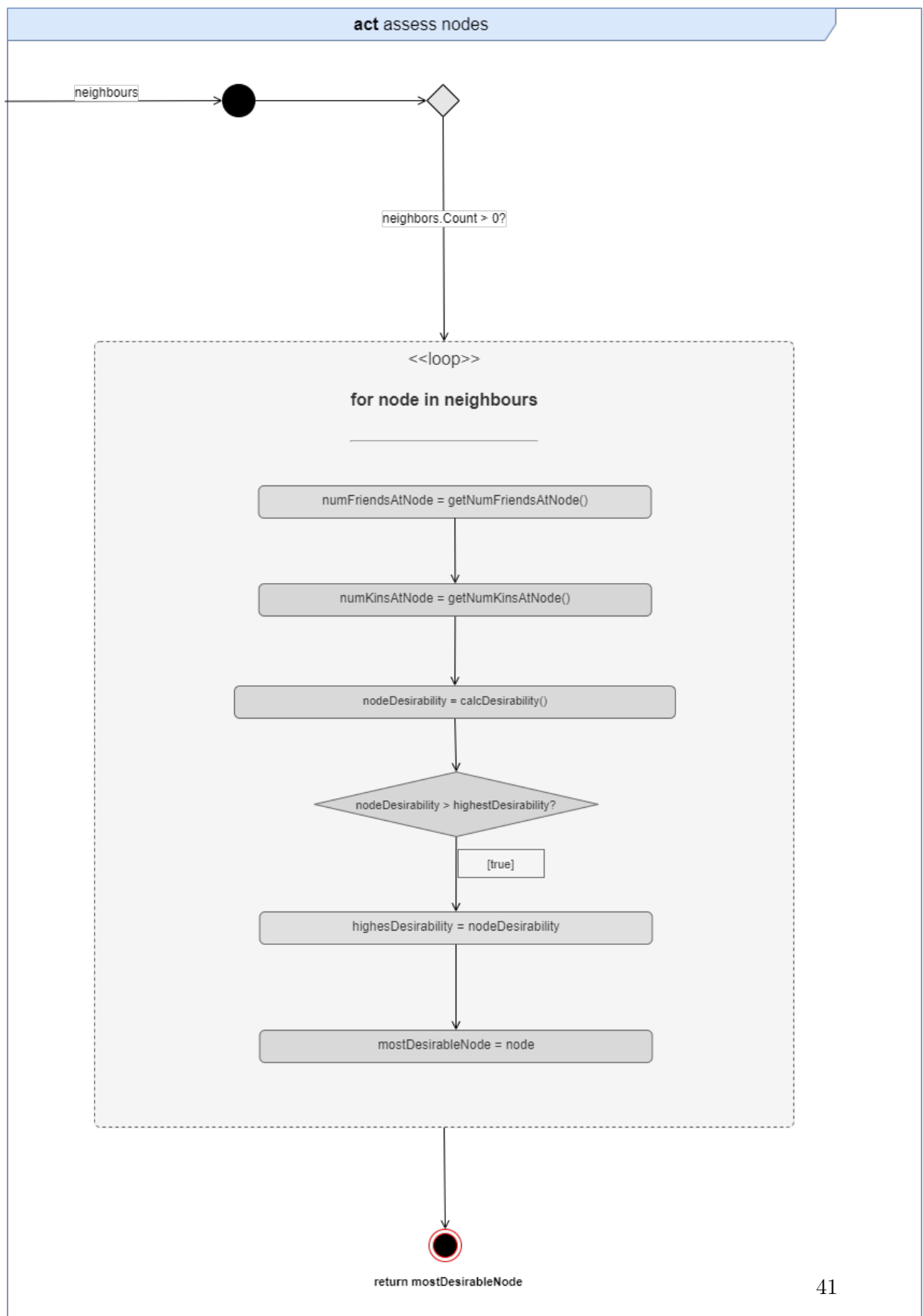
Figure 7.4: Activity diagram showing the algorithm of location assessment
